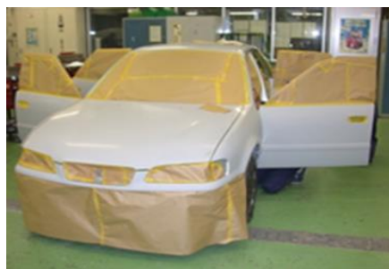
塗装作業(全塗装)
